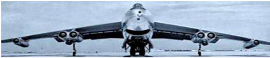
Figure 10.4 Bomber aircraft Boeing B-47 Stratojet with bicycle landing gear
