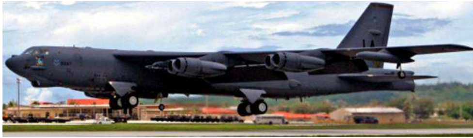
Figure 10.6 Bomber aircraft B-52 Stratofortress with quadricycle landing gear
