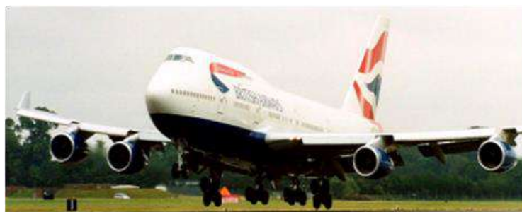
Figure 10.7 Boeing 747 with multi-bogey landing gear
