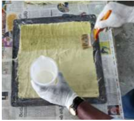
Figure 4.11 Applying Epoxy-Hardener Mixture
