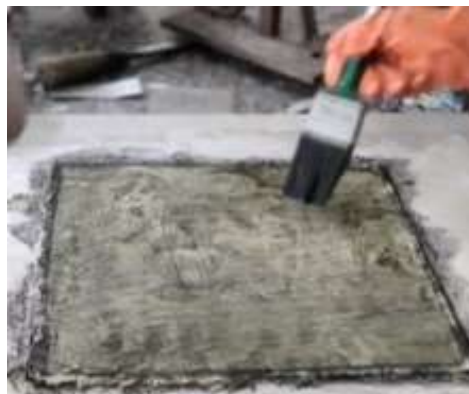
Figure 4.7 Applying Resin + Seashell nanofiller+ MWCNT Mixture on Kevlar plates
