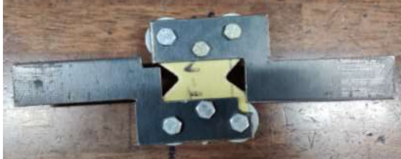
Figure 4.45. Shear Test Specimen fixed in the testing fixture
