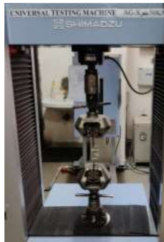
Figure 4.44 Shear testing fixture attached in UTM
