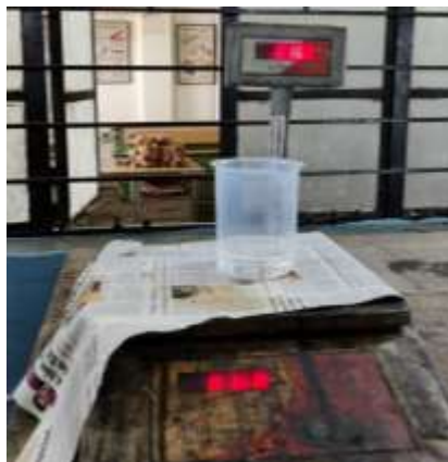
Figure 4.3 Epoxy LY556 measured
