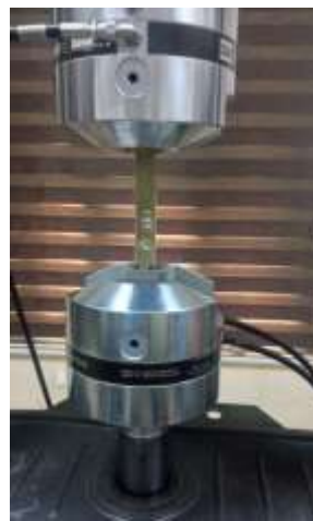
Figure 4.10 Tensile Test Specimen fixed in UTM Fixture
