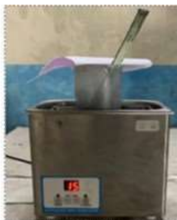
Figure 4.6 Sonification of Epoxy-nanofiller mixture
