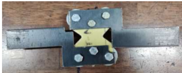
Figure 5.37 Shear Test Specimen fixed in the testing fixture
