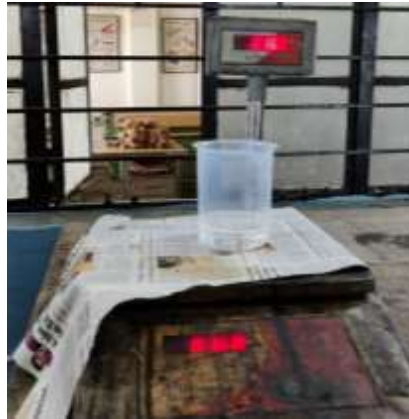
Figure 4.10 Epoxy LY556 measured
