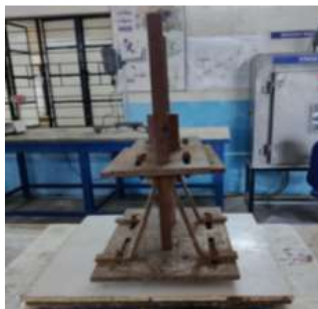
Figure 4.8 Dead weights for curing of composite plates
