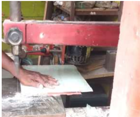
Fig 3.6 Composite is cut using high speed axesaw
