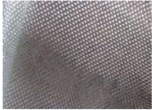
Fig 3.3 Glass fibre of 400 GSM
