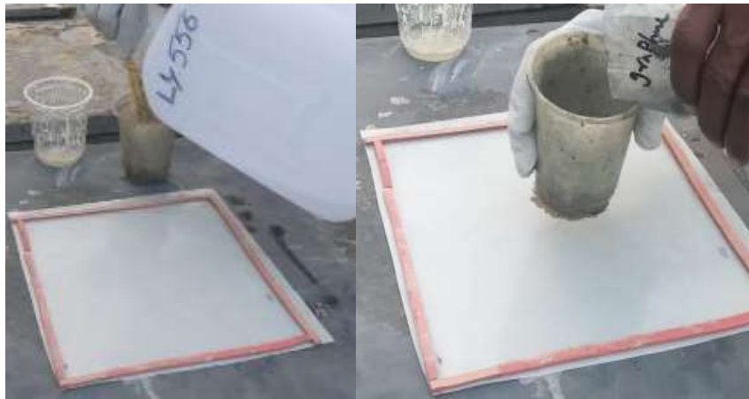
Fig 3.4 Adding Resin and nanofillers
