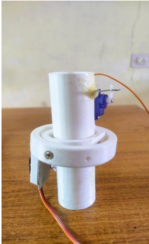
Figure.6.3. 3D Printed Frame of Gimbal mechanism
