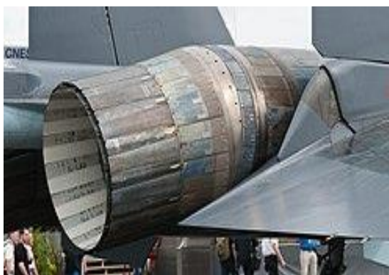
Figure1.1. Thrust vectoring nozzle
