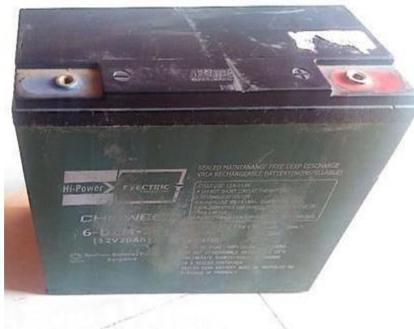
fig 13 Lead acid batter
