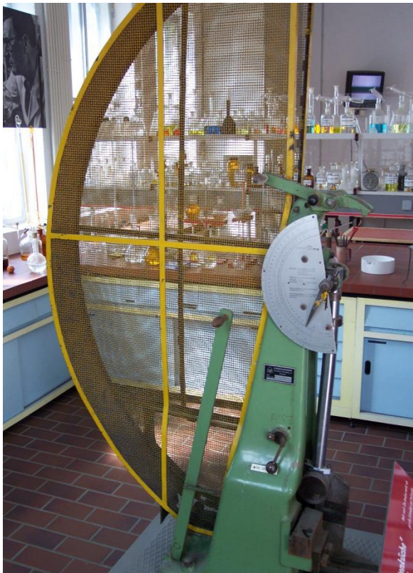
Fig 1.5: Charpy impact test (Wikipedia)
