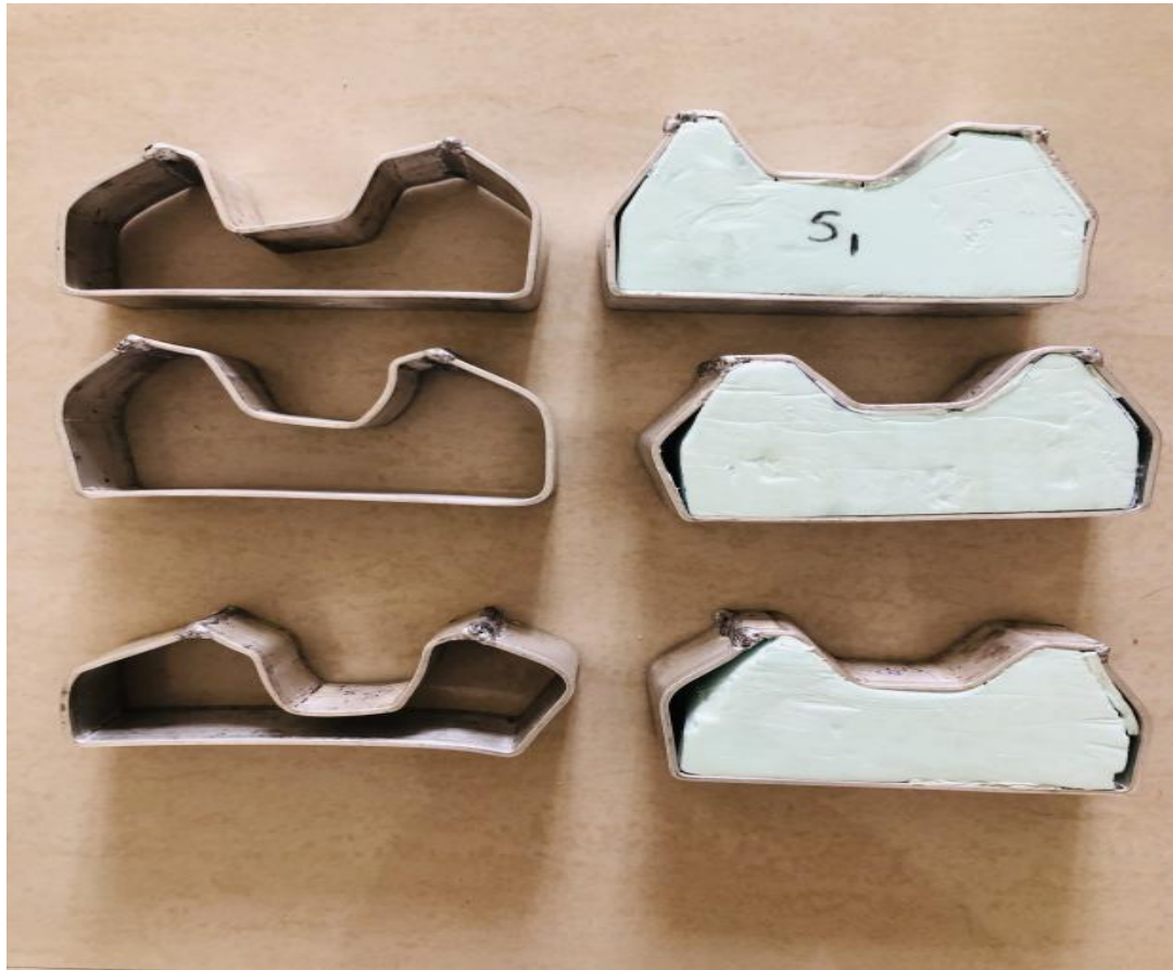
Fig: 7.2 Aluminum 6063 Results - 3mm
