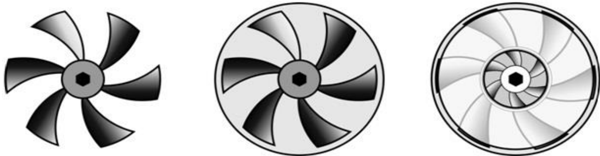
Fig 1.3 : Open, Semi Open, Closed type impellers.
