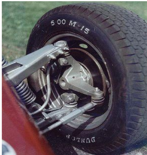
Fig 1.7 A-arms between chassis and wheels
