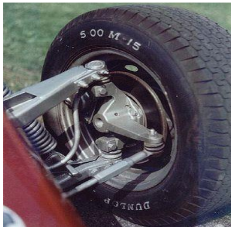
Fig 1.6 Upright held between the A-arms at wheel end
